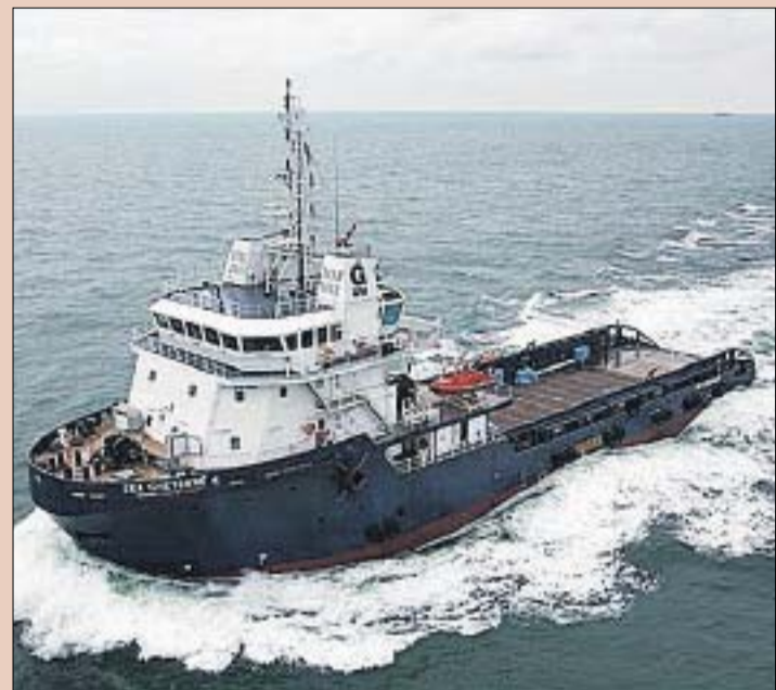
THE "SEA CHEYENNE": One of a series of six 140-tbp AHTS vessels built for GulfMark Offshore by Keppel Singmarine in 2007 and 2008. Fearnley figures show that more than 160 AHTS vessels will be delivered this year.
